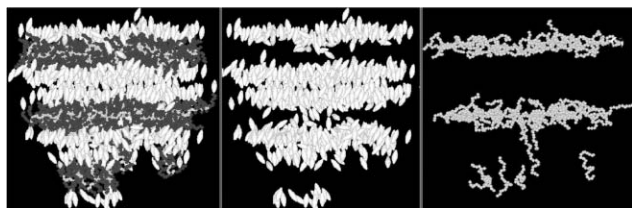
Fig. 5 Top: schematic diagram of a coarse-grained multi-site simulation model for a side-chain liquid crystal polymer. Bottom: snapshots from a simulation of a side-chain liquid crystal polymer showing the formation of smectic liquid crystal layers. 33 The centre and right hand diagrams show a decomposition into mesogenic units and the polymer backbone respectively.
